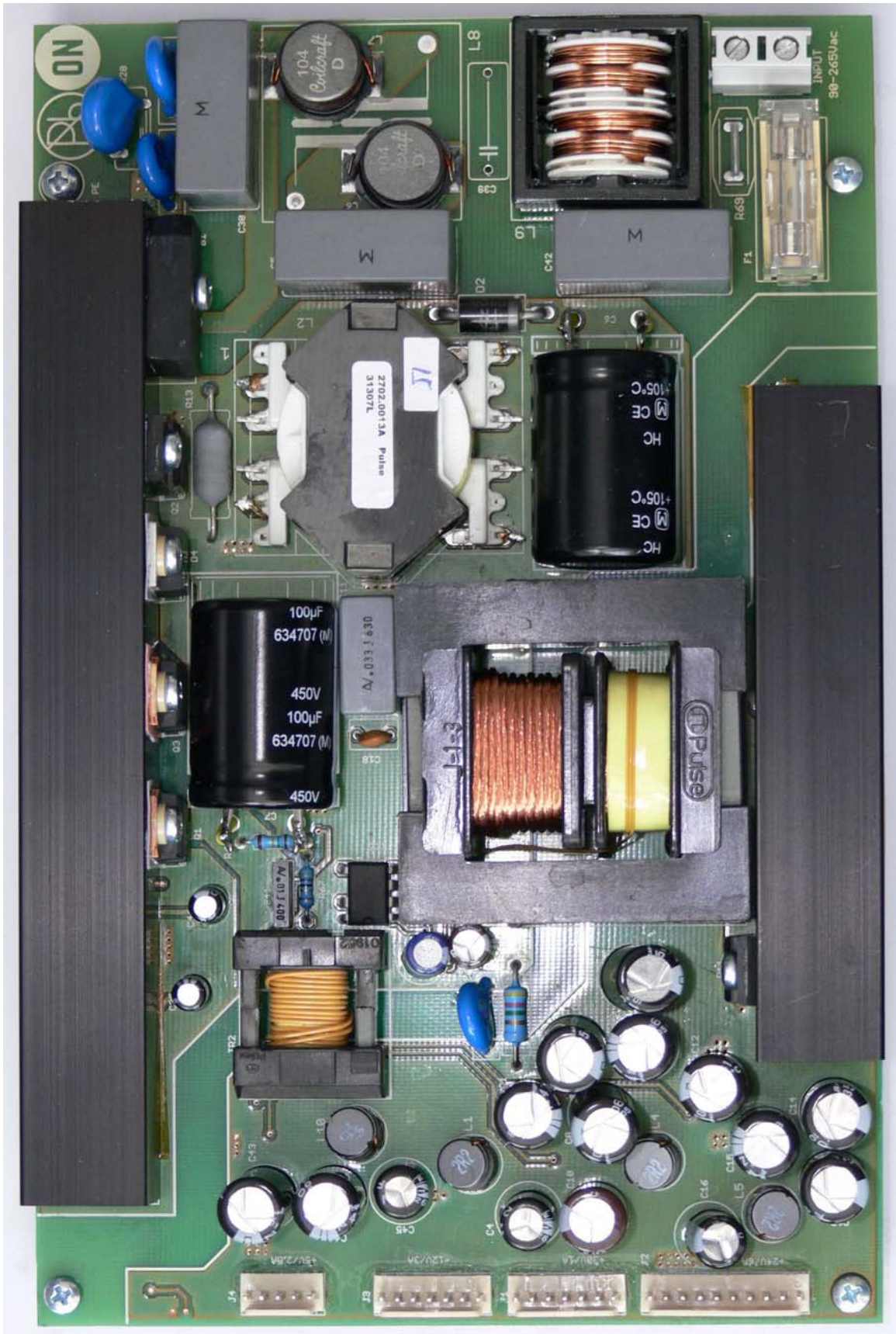
Figure 24. Photo of the Designed Prototype (Real Dimensions are 200 x 130 mm)
